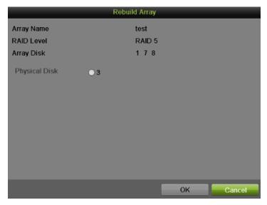
Figure 141 Rebuild Array Interface
